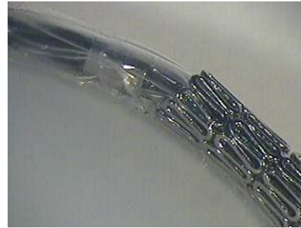
Figure 3: Proximal stent end while bended over a 7.5 mm radius; distance between outer contours d=120 \mu\text{m} , Medtronic AVE S7 3.0/15 mm
