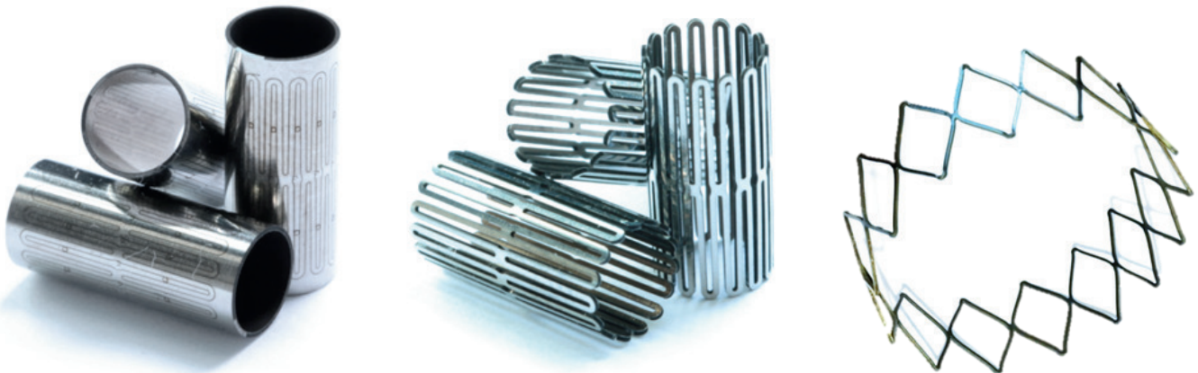
Process steps for the fabrication of stent structures using femtosecond laser cutting – from cutting of tube semi-finished products through mechanical post-processing to shape setting by heat treatment
