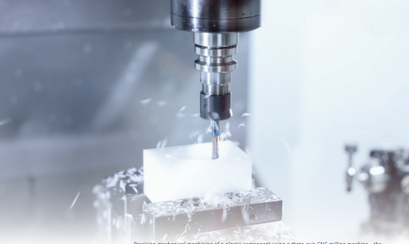
Precision mechanical machining of a plastic component using a three-axis CNC milling machine – the technical implementation at IIB e.V. is carried out by experienced electronics and software engineers as well as designers and precision mechanics.
